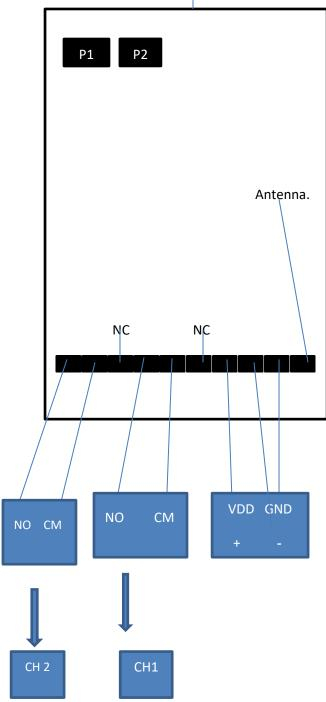
Working voltage: 12-24V Frequency: 433.92MHZ
