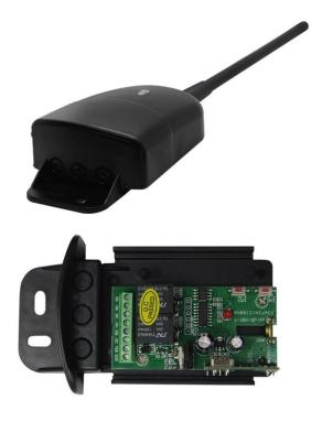
Working voltage: 12-24V Frequency: 433.92MHZ
