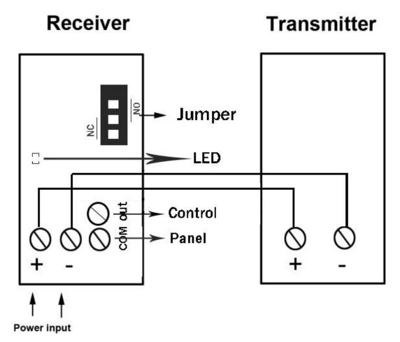
After you have completed wiring, check the alignment between transmitter and receiver to ensure the photocells work efficiently. Power on after the correct wiring, the user will find the LED indicator will light up (set N.O. through jumper) or goes out (set N.C. through jumper) when the units are correctly aligned.
