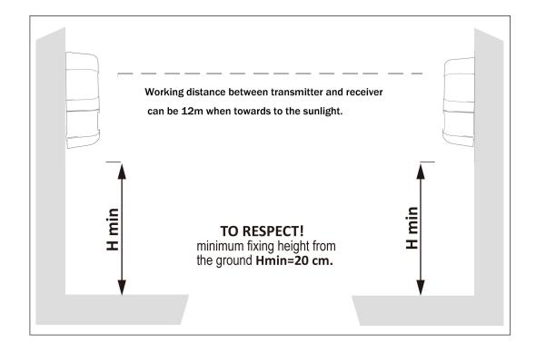
The user should install the photocells on the back of the direct sunlight or other strong light source to keep it working steadily.
